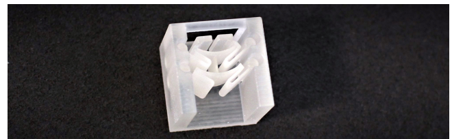
Figure 22: A cell printed fully assembled using shapeways' “frosted detail plastic” material.
