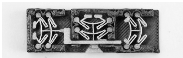
Figure 10: We cross signals by running a crossbar across another cell.
